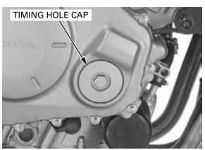
Turn the crankshaft clockwise, align the "T" mark on the starter clutch outer with the index notch on the right crankcase cover.
